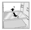
**SHELVES**: with or without grill. Due to the special guides the shelves are removable and the height is adjustable (*see diagram*), allowing easy storage of large containers and food. Height can be adjusted without complete removal of the shelf.
